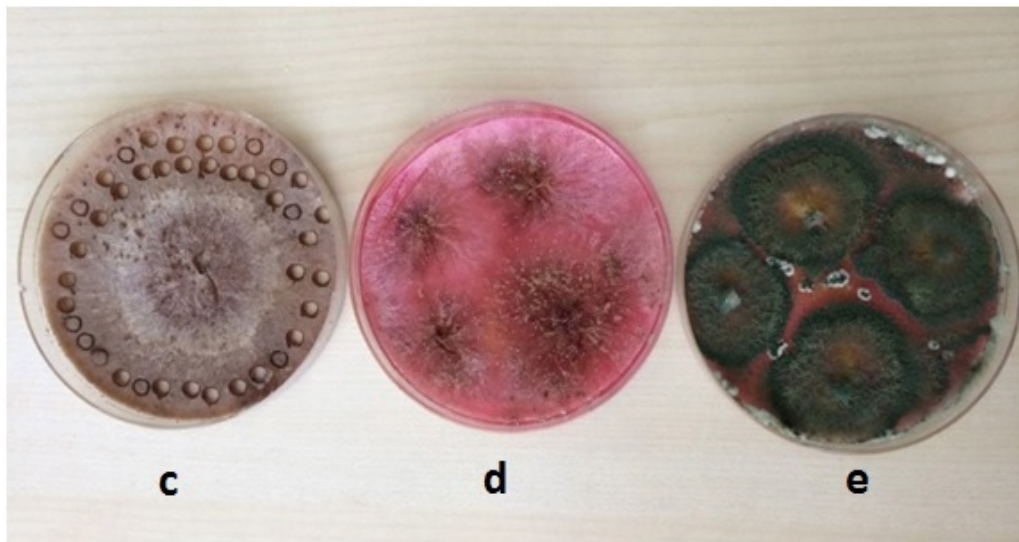
Figure 2. Discs cut from thoroughly washed colony (c), rapid growth of Rhizoctonia solani alone on PDA having Rose Bengal and Streptomycin (d), growth of mycoparasites on the same medium having additionally tolclaphos-methyl (e).
